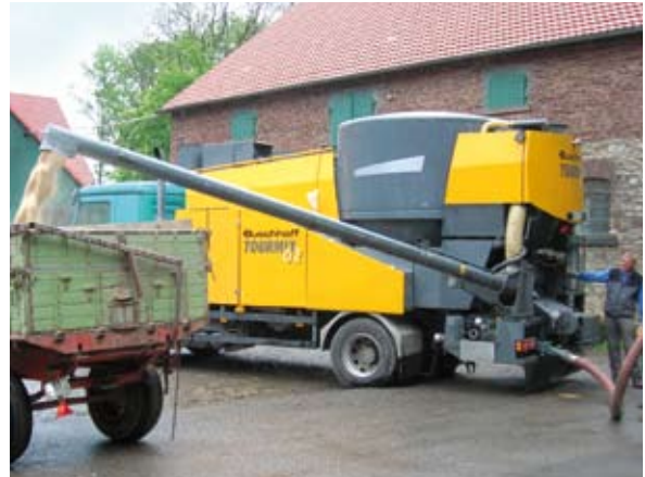
TOURMIX 02-VE with direct drive during continuous grinding
